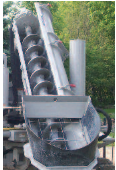
Auger Conveyor; lid opens for cleaning.
