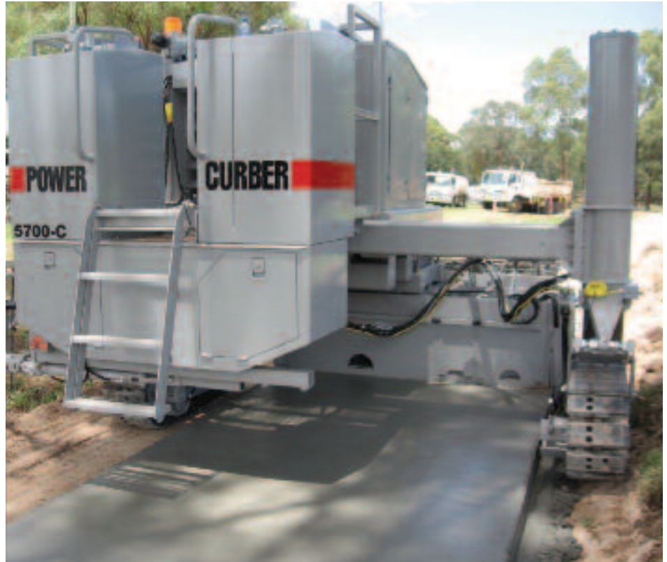
Center pour paving 6.5' (2m) wide in Australia. Optional polyurethane pads are shown.
