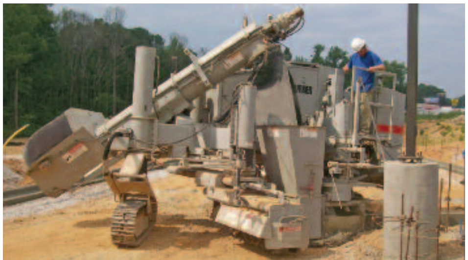
Front track steering (pictured) is standard. All crawler steering is optional.
